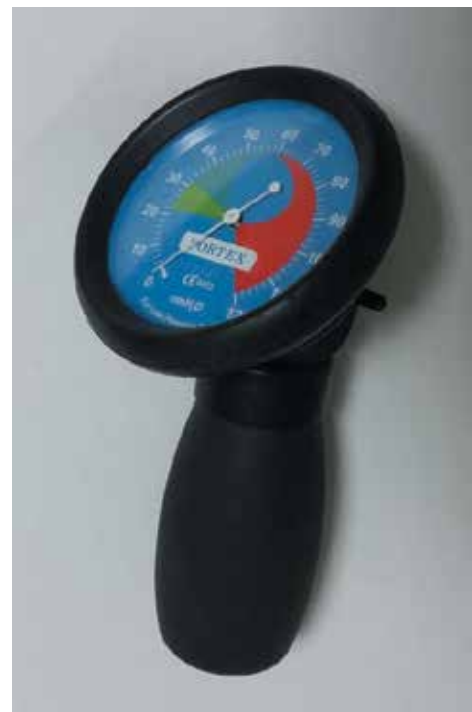
Figure 4: Endotest by Portex; for checking endotracheal tube cuff pressure. Permissible upper limit is around 30 cmH 2 O, which is capillary pressure in tracheal mucosa. Excessive pressure may be a source of postextubation cough, but it is definitely linked to subglottic stenosis due to ischemic changes.
