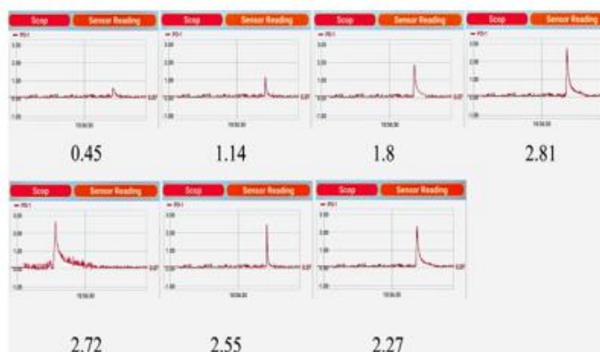
Figure 4. Effect of Luminol volume on CL intensity
